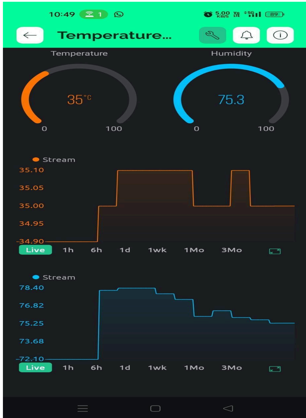
Fig 2.6 The Temperature and Humidity data are Being Displayed on the Blynk Mobile Application
