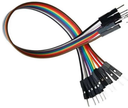
Fig:2.9: Jumper Wires
