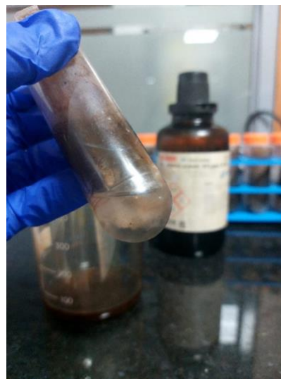
Fig 4.5 Centrifugation process Fig 4.6 Separation of Graphene oxide from supernatant
