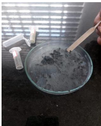
Fig 4.9 Scraping dried Graphene oxide Fig 4.10 Storage of Graphene oxide
