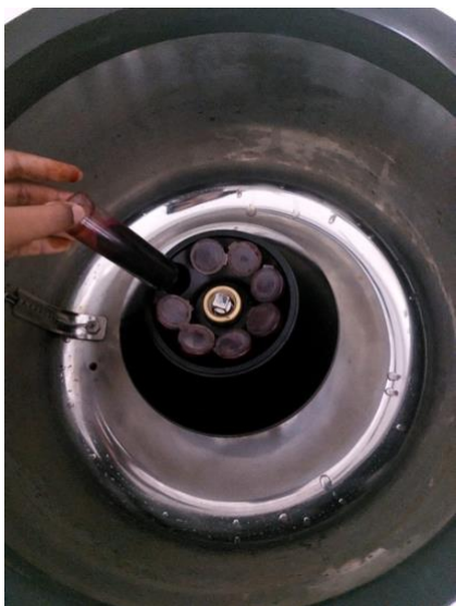
Fig 4.5 Centrifugation process Fig 4.6 Separation of Graphene oxide from supernatant
