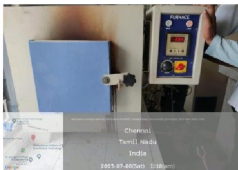
Figure 4.4: Calcination of waste chicken eggshell powder
