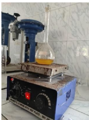
Figure 4.13: Transesterification is placed in magnetic stirrer of Jatropha curcas oil
