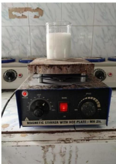
Figure 4.5: CaO is incorporated in deionized water
