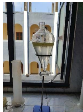
Figure 4.15: Water washing of methyl ester
