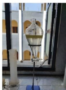
Figure 4.15: Water washing of methyl ester
