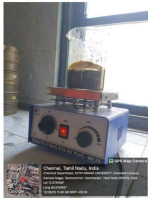
FIG:4.4 Acid activation for siam weed
