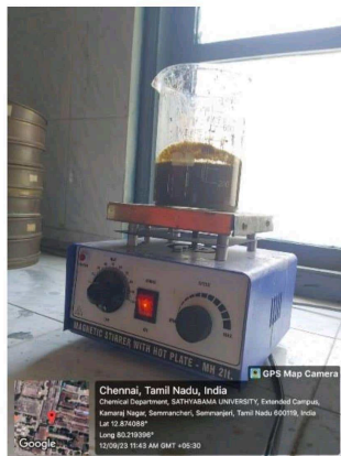
Fig 4.4 Acid activation for siam weed
