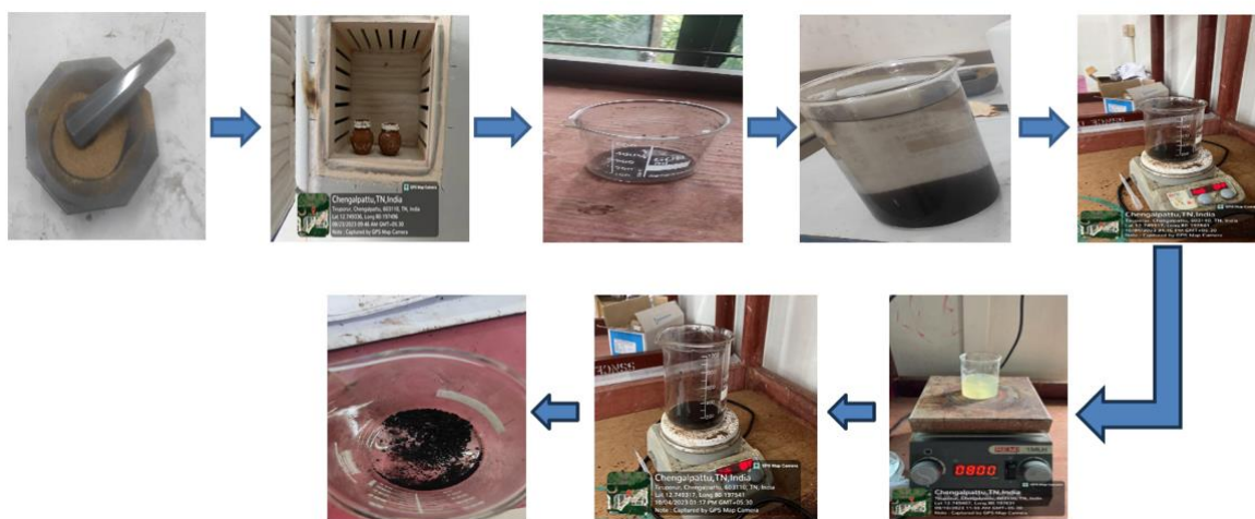
Fig:4.1: Step by step procedure Chitosan coated Sargassum Wightii Biochar (CSWBC) biochar derived Sargassum Wightii
