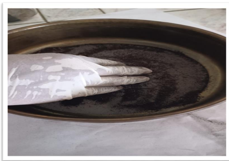
Fig. 4.3 Sieving of sugarcane Bagasse powder.
