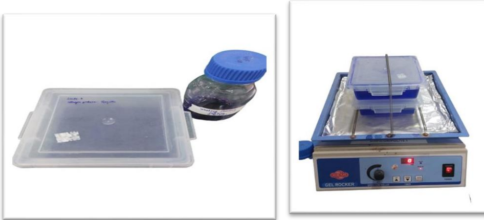
Fig 4.3.3.4 Staining of Acid Soluble Collagen of Sphyraena obtusata and Psettodes erumei In gel rocker
