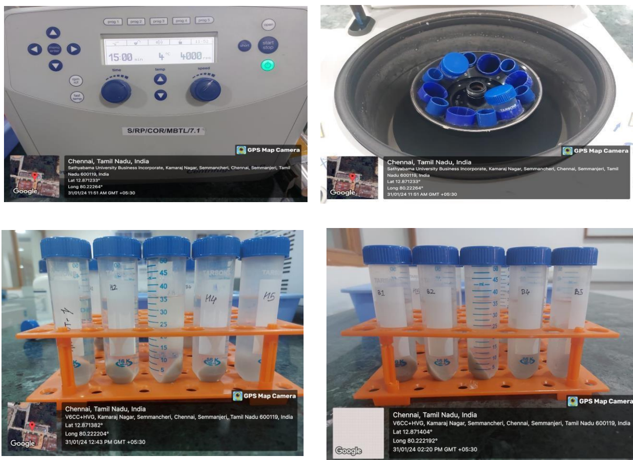
Fig 4.3.5 Centrifugation of Acid soluble Collagen Sphyraena obtusata and Psettodes erumei .
