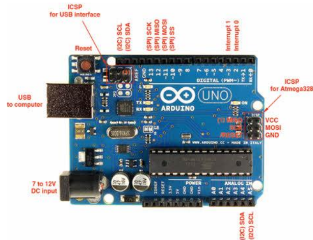
FIG- 4.6 Arduino Uno Board Pin Configuration
