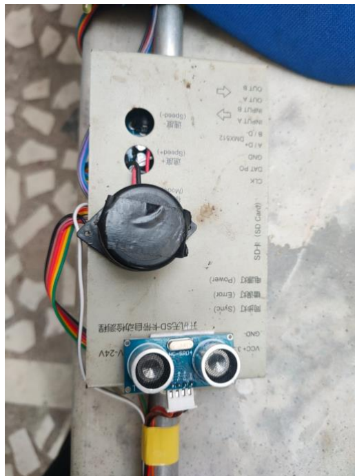
Fig;5.6 Ultrasonic Sensor, LIDAR, The Box contains an Arduino Nano
