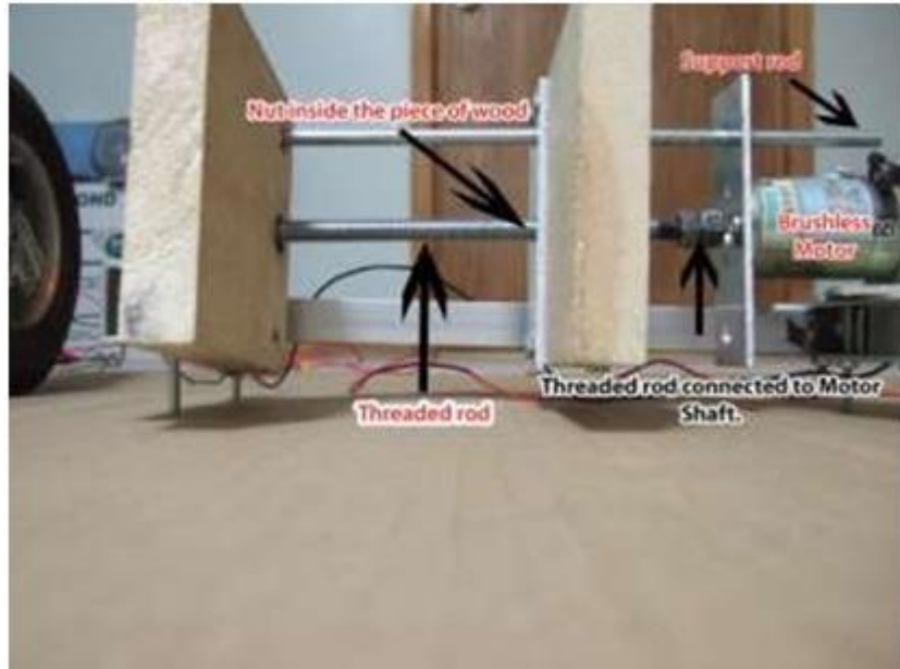
Fig 4.4: Lifting using threaded shaft
