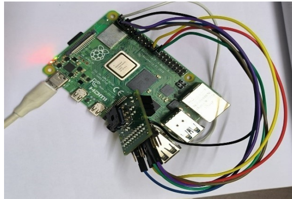
Fig: 4.4: Infrared camera module with complete wiring
