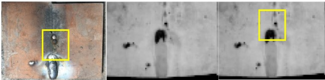
Fig:5.1: Welded metal with spatter defect
