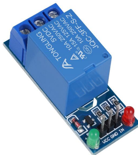
Fig:4.9: Relay Board
