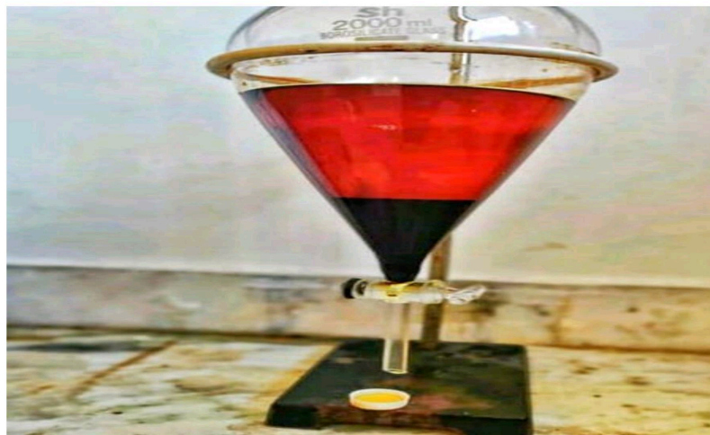
Fig: 4.5: Extraction of bio-diesel from waste cooking oil
