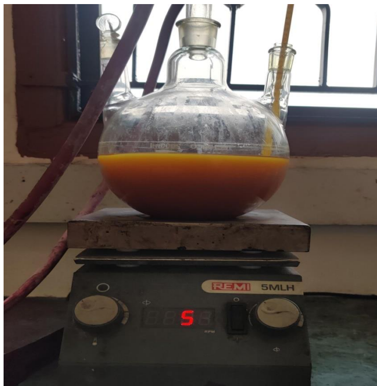
Figure 10: Transesterification of FFA in bio diesel
