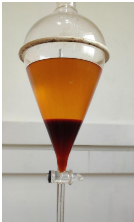
Figure 13. Water wash for bio diesel of production in FFA
