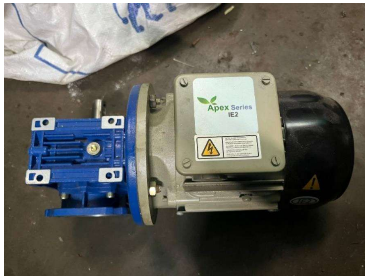
Fig 4.2: 0.5hp 3 Phase Squirrel Cage Induction Motor
