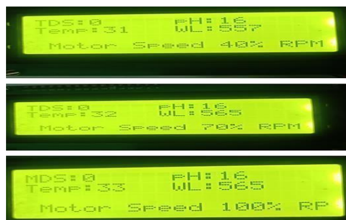
Figure 4.9: LCD Display for Fan Speed Control Based on Sump Water Temperature
