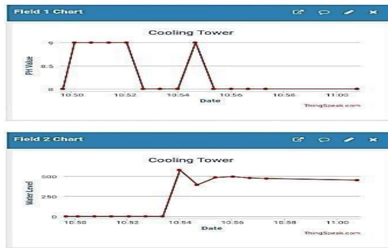
Figure 4.12: IoT Screen Monitoring pH and Water Level Fluctuations
