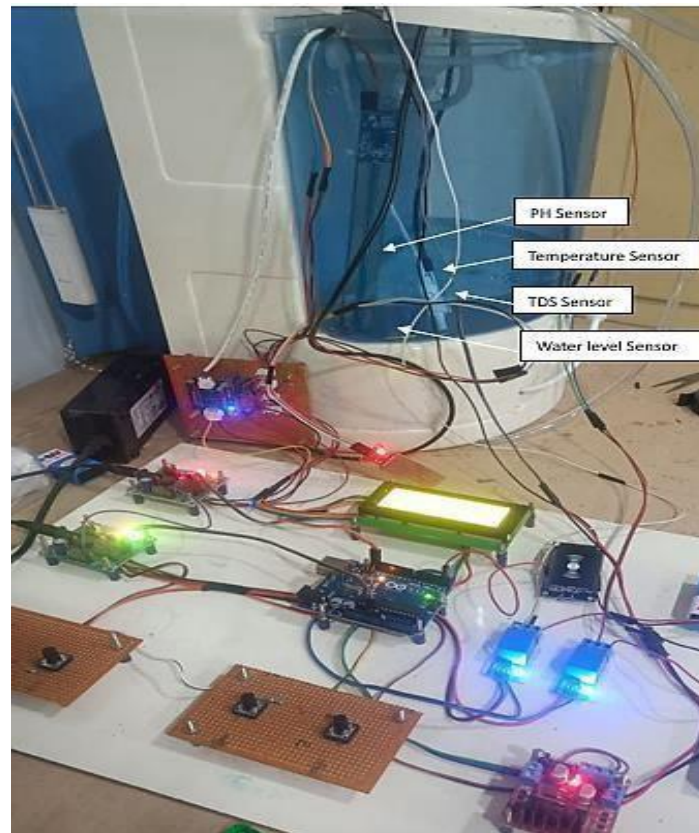
Figure 4.7: Layout of Sensors Inside the Cooling Tower
