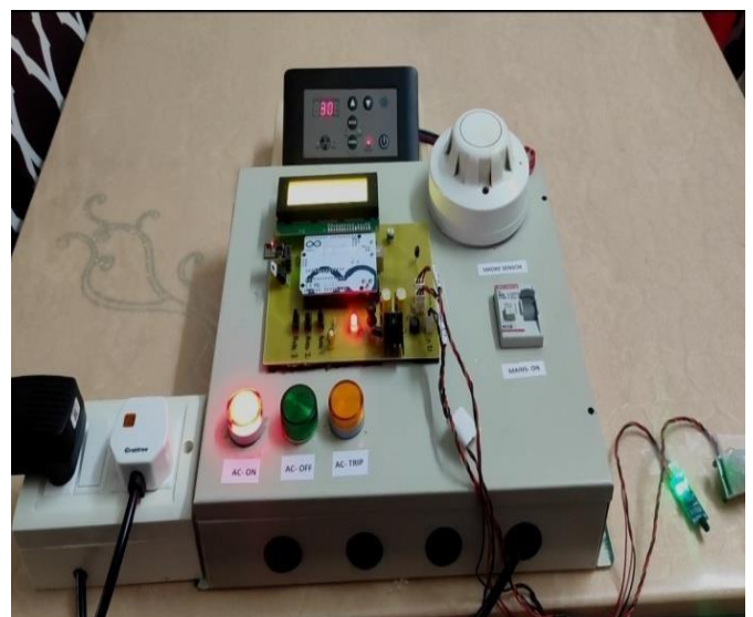
Fig. 9. AC compressor switches on after 3 minutes
