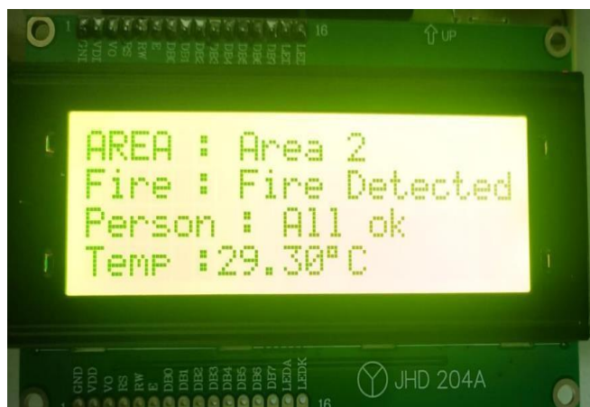
Fig. 12. LCD shows fire detected in IoT module
