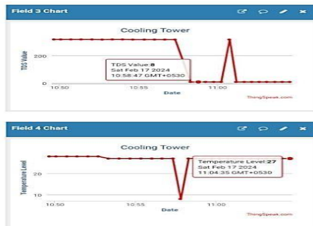
Figure 18: IoT Screen Monitoring TDS and Water temperature Fluctuations
