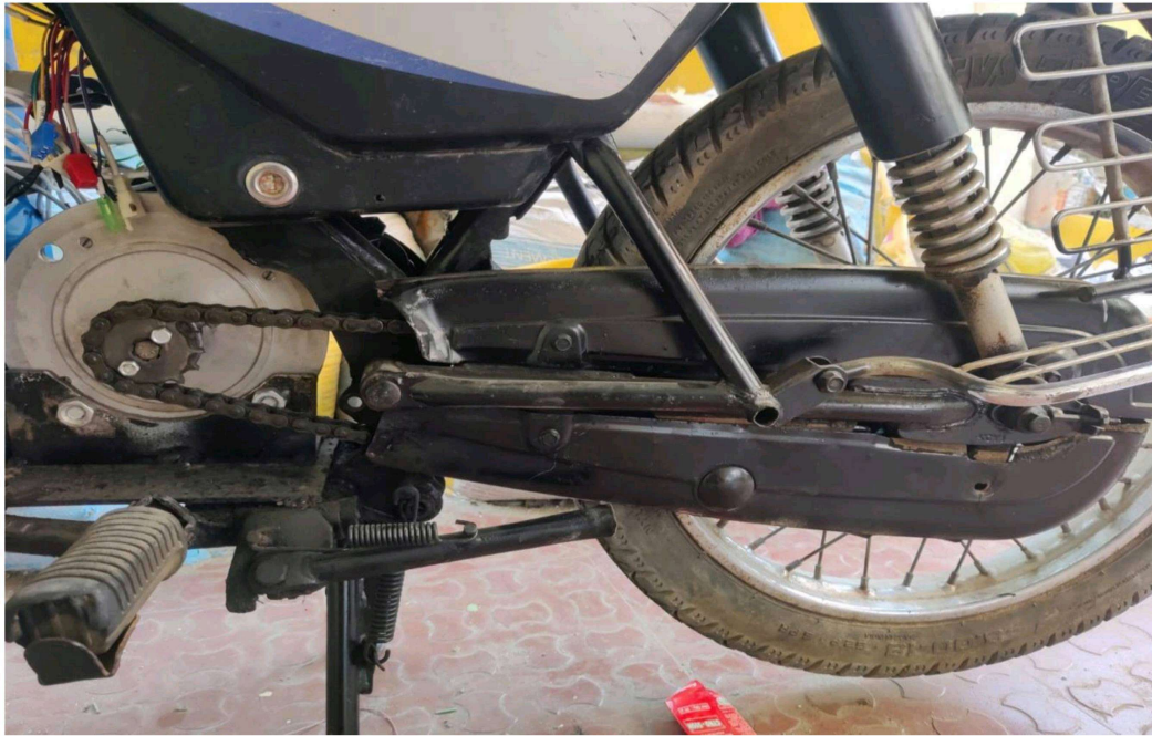
Fig.4.9 Chain Drive to Wheel
