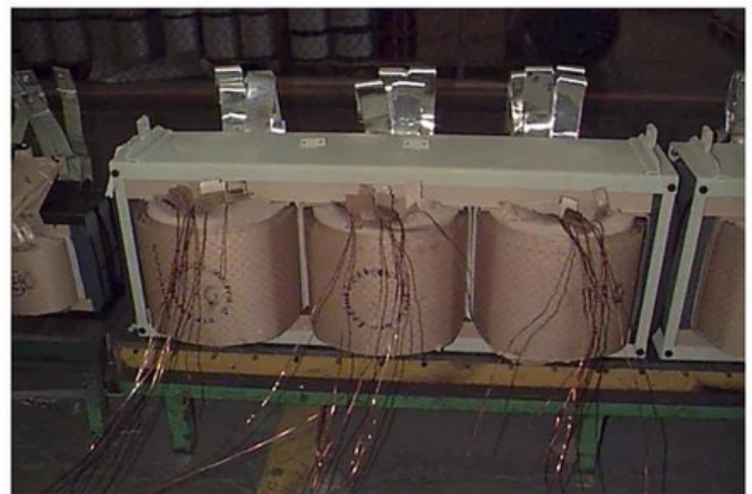
fig no 2.4 Coil of the transformer
