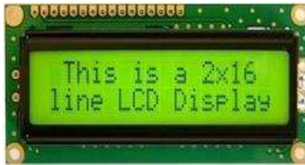
Fig 4.5: 2x16 Line Alphanumeric LCD display
