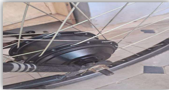
Figure 6.1 After installing hub motor
