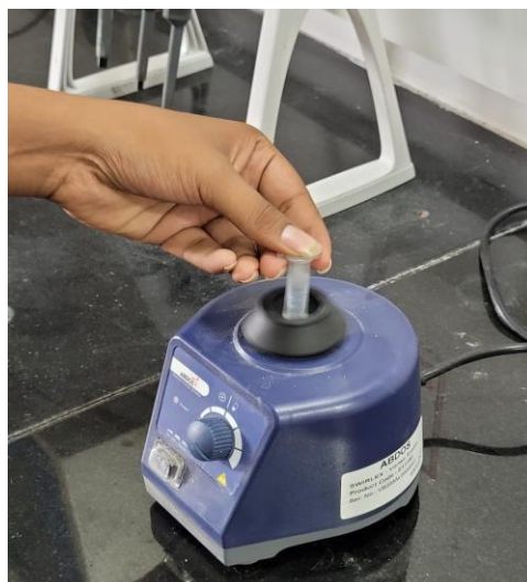
Fig 4.3 Stirring of a mixture of polystyrene, chloroform, and graphene
