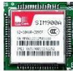
Fig 3.5 SIMCom SIM900AGSM Module
