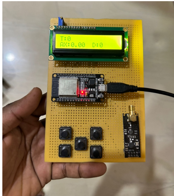
Fig: 5.3: RC boring machine Remote control unit with data shown
