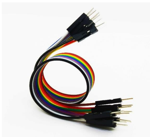
Fig: 4.7 : Connecting Wires
