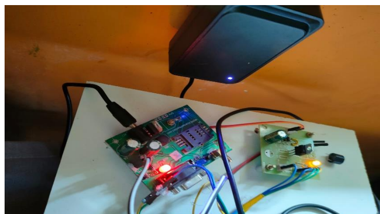
Fig:5.5 Power supply to the GSM modem.
