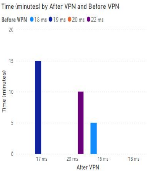
FIGURE 11: Time Latency shows latency measurements (in milliseconds) at various time intervals (0, 5, 10, 15 minutes) for a network before and after the implementation of a VPN. Before VPN, latency ranged from 18-22 ms, while after VPN, it improved slightly, with latency ranging from 16-20 ms.
