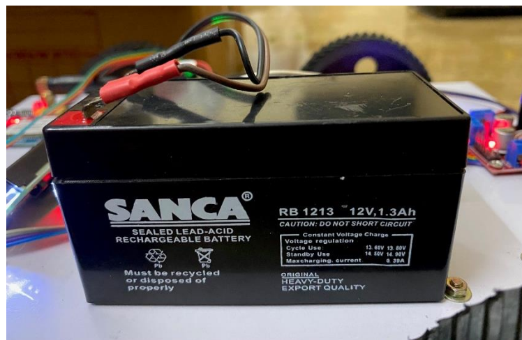
Figure 4.9 12V/1.3AH Sealed Lead Acid Battery
