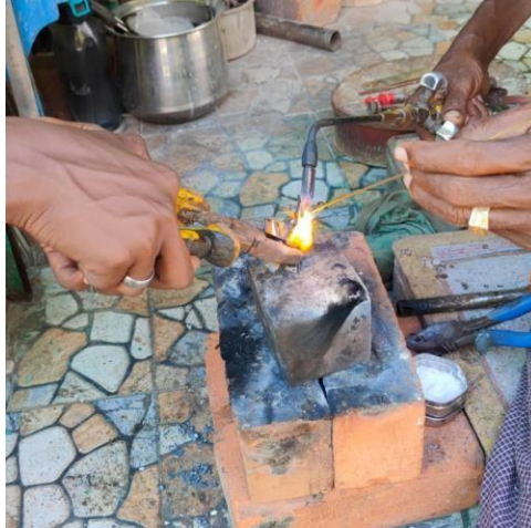
Fig:4.3 : Brazing of Compressor
