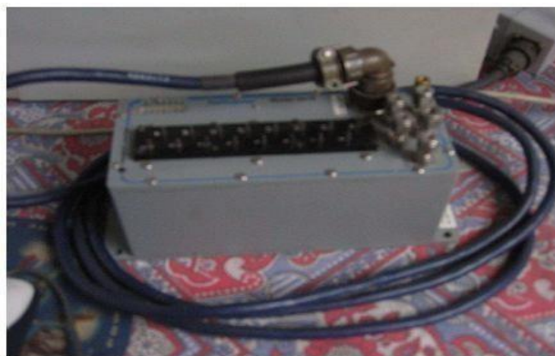
Fig: 6.3 : PSI Model 9016 16 Channel Pressure Transducer
