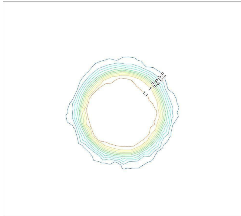
Fig:5.28 : Isomach contour of circular nozzle at X/D=0
