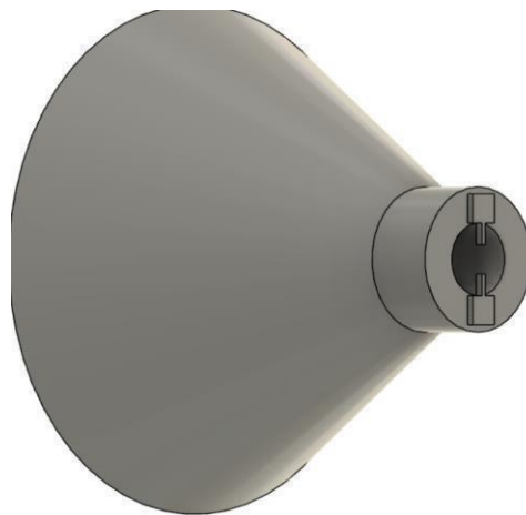
Fig: 4.8 : Nozzle with tab (AR 10)
