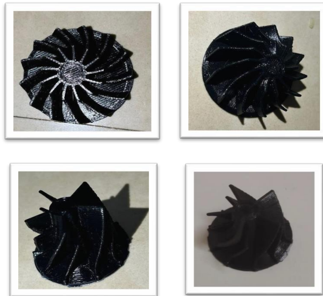
Fig:5.7 : 3D Printed Impeller
