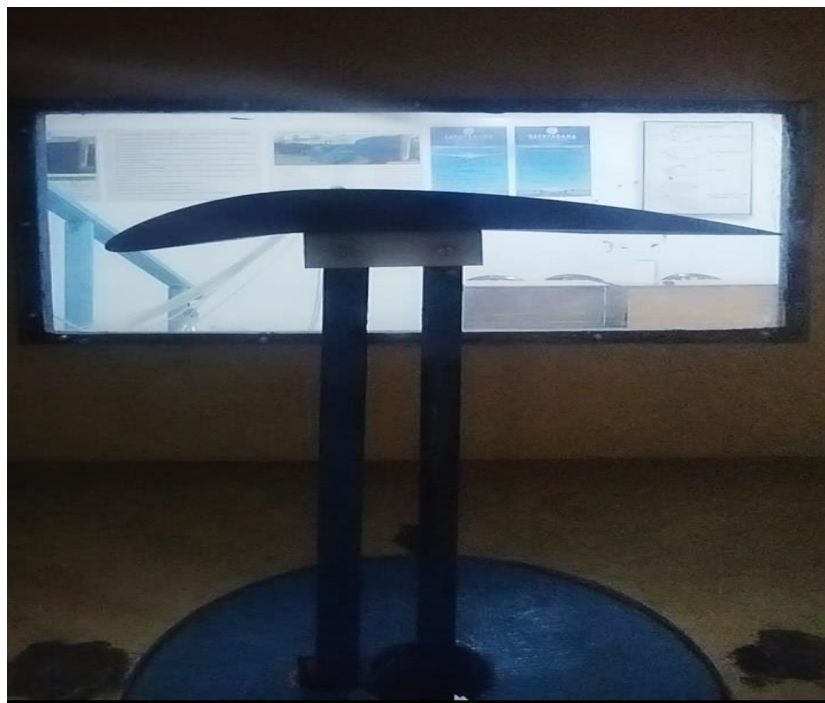
Fig:4.20 : Testing of Plain Wing in Wind Tunnel
