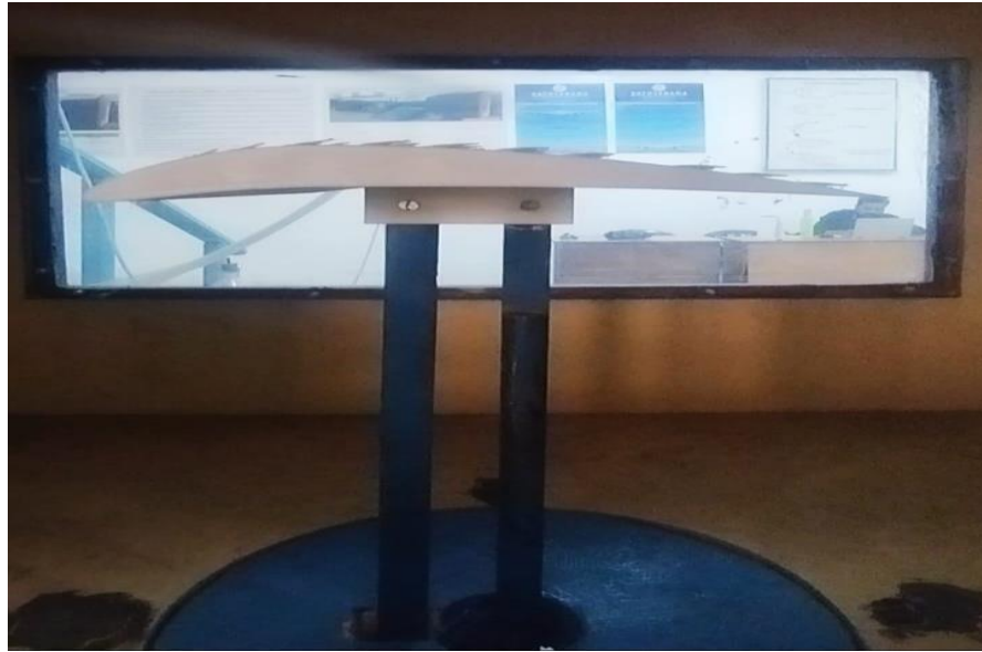
Fig:4.21 : Testing of Wing with Denticle in Wind Tunnel
