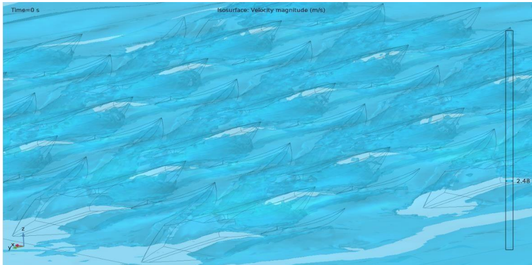
Fig:5.2 : Simulation of Denticle matrix in a flat plate
