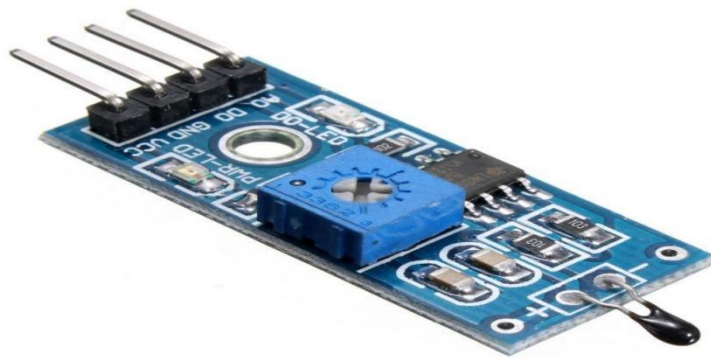
Fig:4.4: Temperature sensor.
