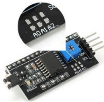
Fig:4.8 : Address selection pads in the I2C-to-LCD piggy-back board
