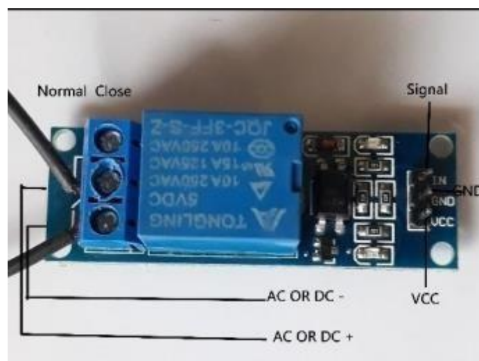
Fig.4.4 Relay as Controlling unit
