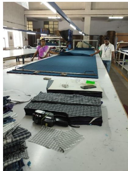
Fig 17 Laying the fabric
