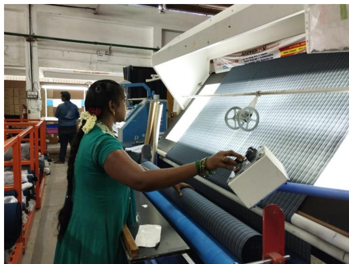
Fig 9 Checking the fabric
