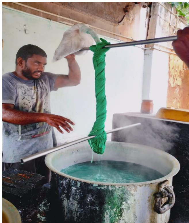
Figure 74 Draining the water by twisting
