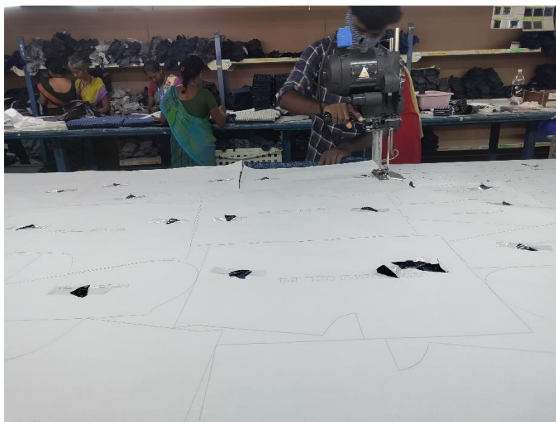
Figure 30 ( cutting the layed fabric with straight knife cutting machine )
