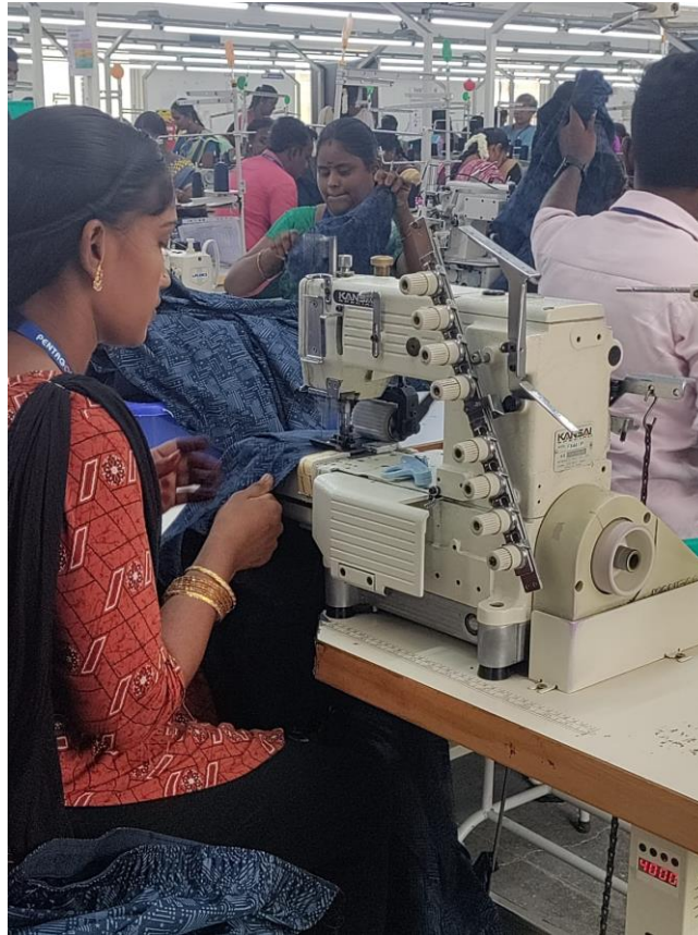
Figure 37 ( attachment of elastic to the garment )
