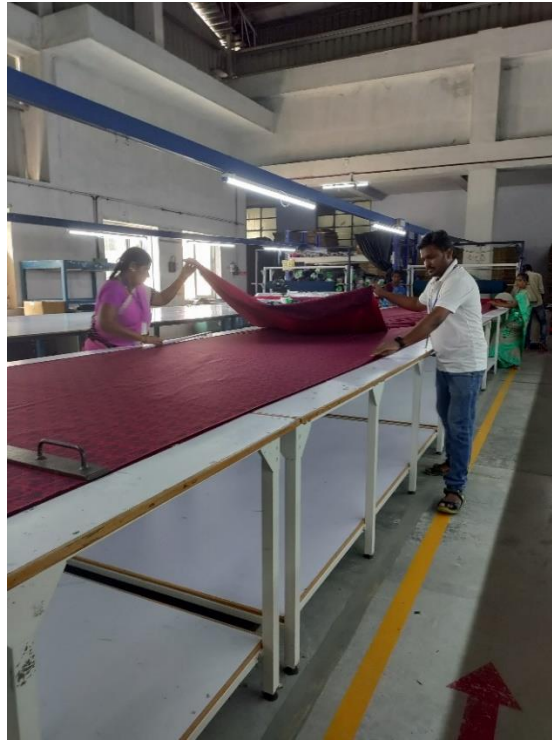
Figure 22 ( fabric laying for cutting )
