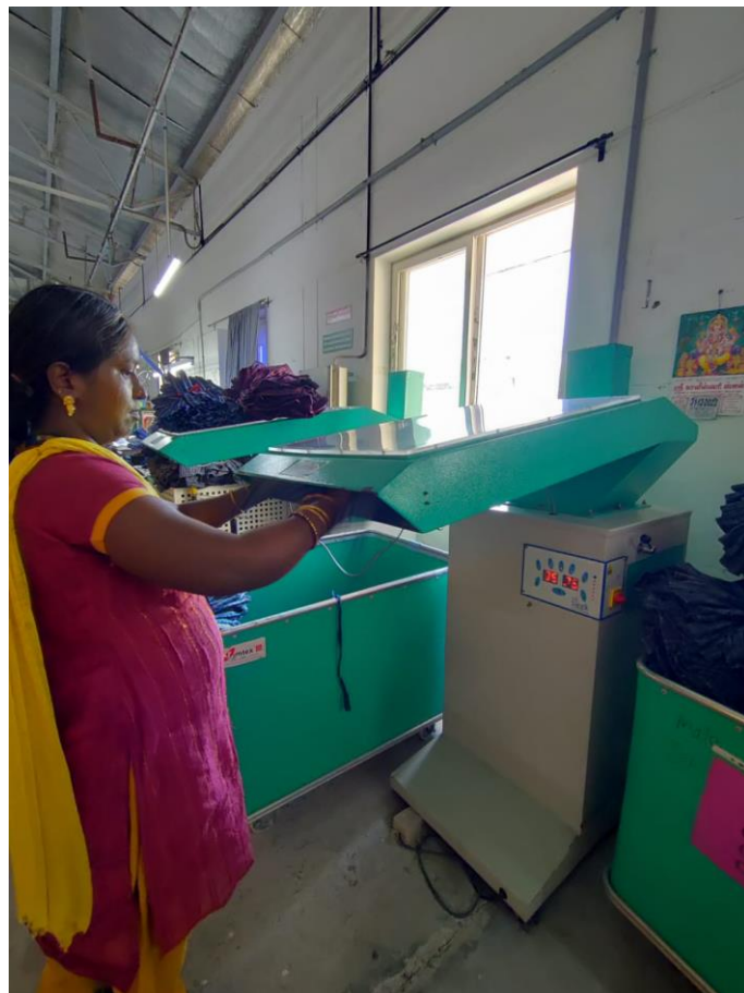
Figure 44 ( removing of excess thread by thread sucking machine )
