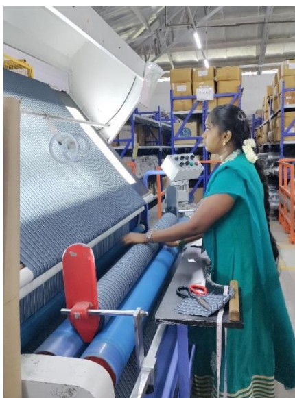
Figure 13 ( inspection of fabric before cutting )
