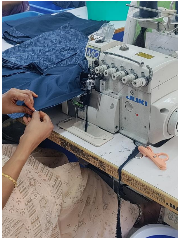
Figure 35 ( over-locking at side seams )
