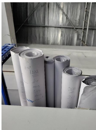
Figure 24 ( PATTERNS MARKED IN SHEETS FOR CUTTING )
