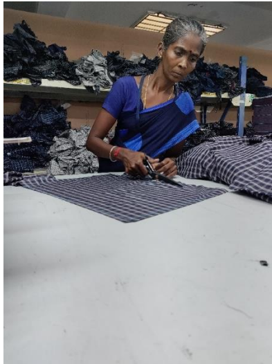
Figure 29 ( recutting of the defected fabric piece manually )
