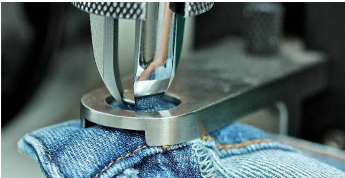
Figure 33 – Button pulling test
