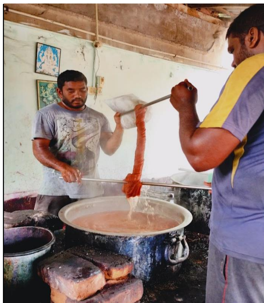
Figure 71 Draining the water by twisting
