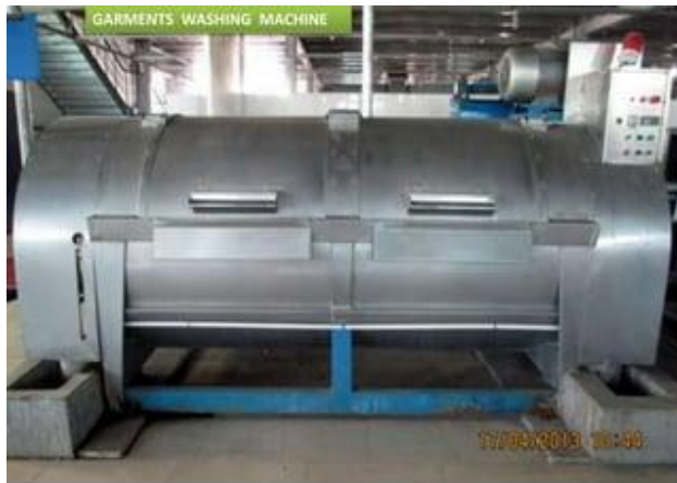
Figure. 38 Washing Machine. Washing typically occurs following garment sewing.
