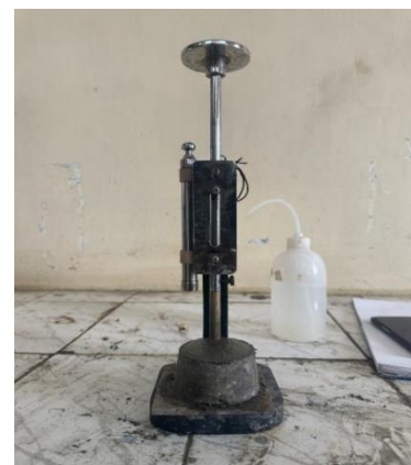
Figure 4.19 Test for consistency
