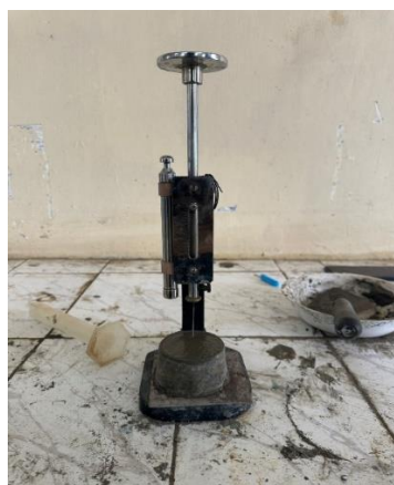
Figure 4.20 Needle penetration test
