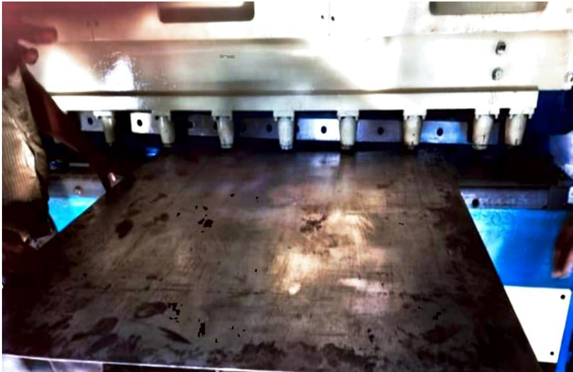
Fig 3.2: Machine Cutting of CR Sheet
