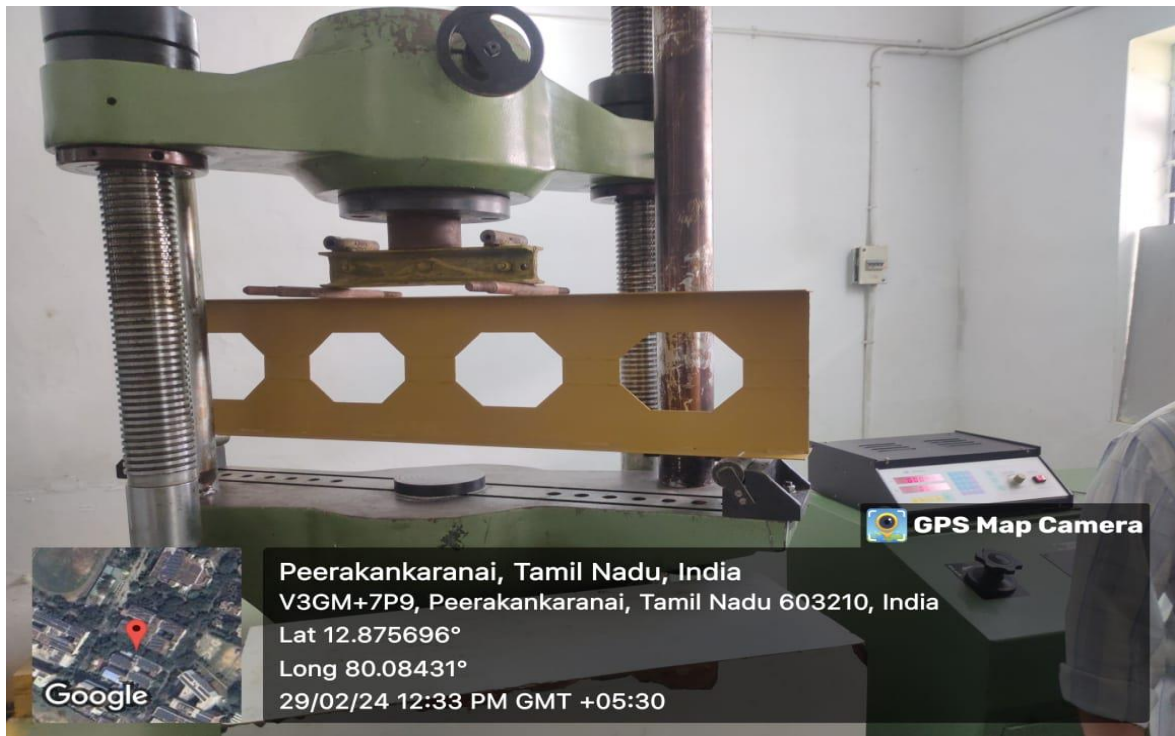
Fig 3.30: Testing Set-Up of CRCB-2
