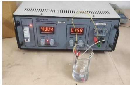
Fig: 4.5: Anodic \text{TiO}_2 Nanotubes Fabrication
