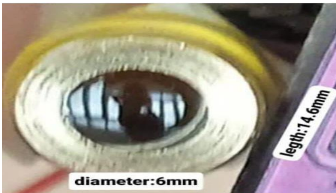
Fig:4.7: Laser diode used in DCS probe
