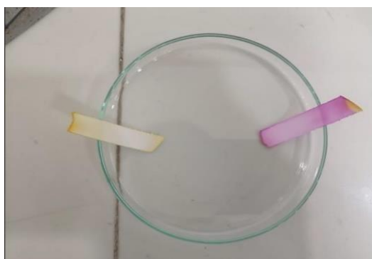
Fig. 4.8 Phenol red reaction on dehydrated (left) and rehydrated (right) sample
