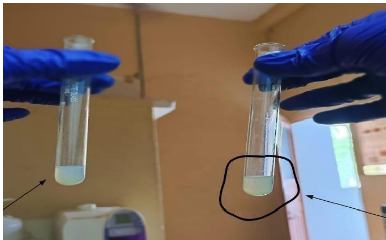
Fig. 4.4 Increased coloured turbidity indicating presence of more chlorine concentration
