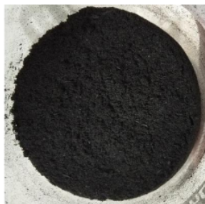
Fig 1.6 Biochar produced from wood bark of Neem
