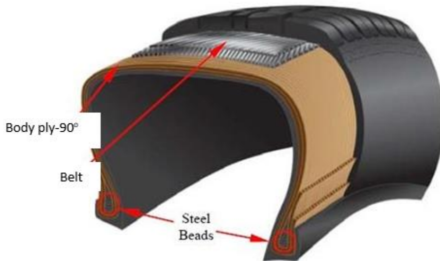
Figure 1 Radial Body ply & Belt
