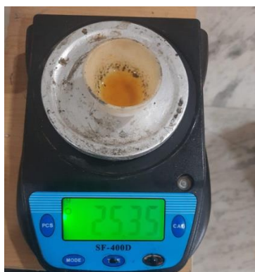
Fig 5.4 Oil sample after 110 C in hot furnace
