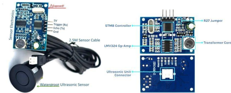
Figure 5.3 AJ- SR04M and Circuit board
