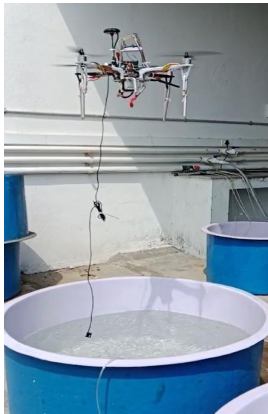
Figure 6.2: Sensor transducer measuring water depth from drone
